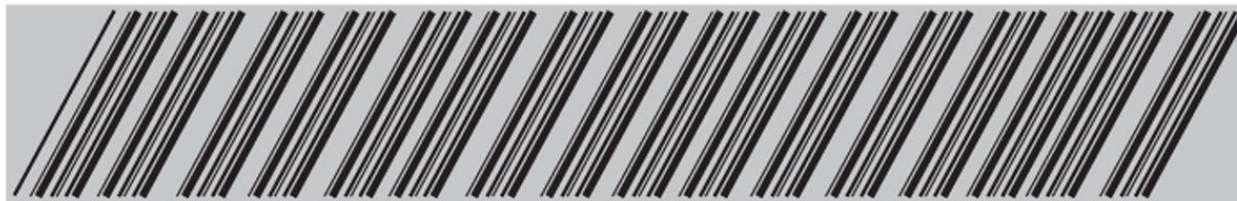
Helical scan tape format
