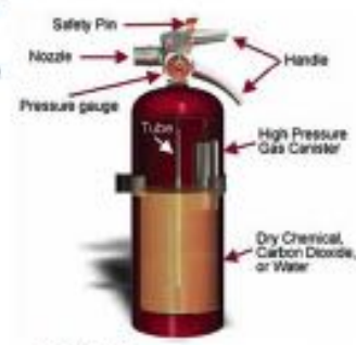
FIGURE 1 How a fire extinguisher works
